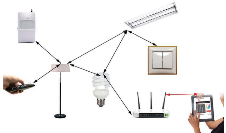
Fig. 1: Low-power wireless lighting control.
